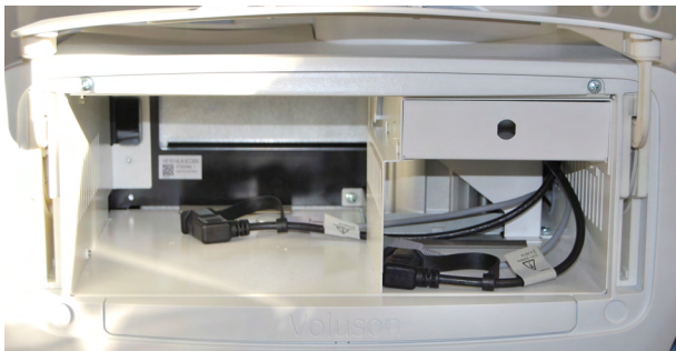
The outlet voltage is set to 115V~ independent from the supply mains voltage.
